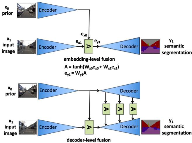
Figure 2. **Network Architectures.** A compact encoder-decoder network architecture is used with the addition embedding-level (top network architecture) and decoder-level (bottom network architecture) prior fusion. Prior features are combined using  $\tanh$  activation functions, similar to those in recurrent networks.
